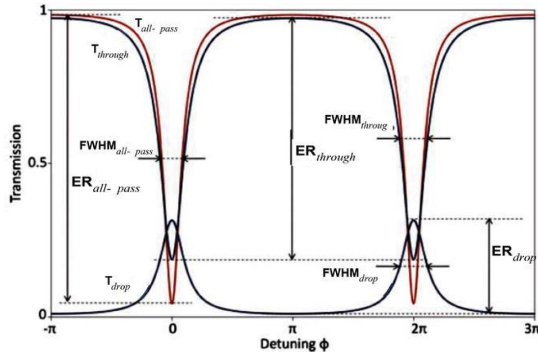
Transmission spectrum of an all-pass ring and the two outputs of add-drop ring
