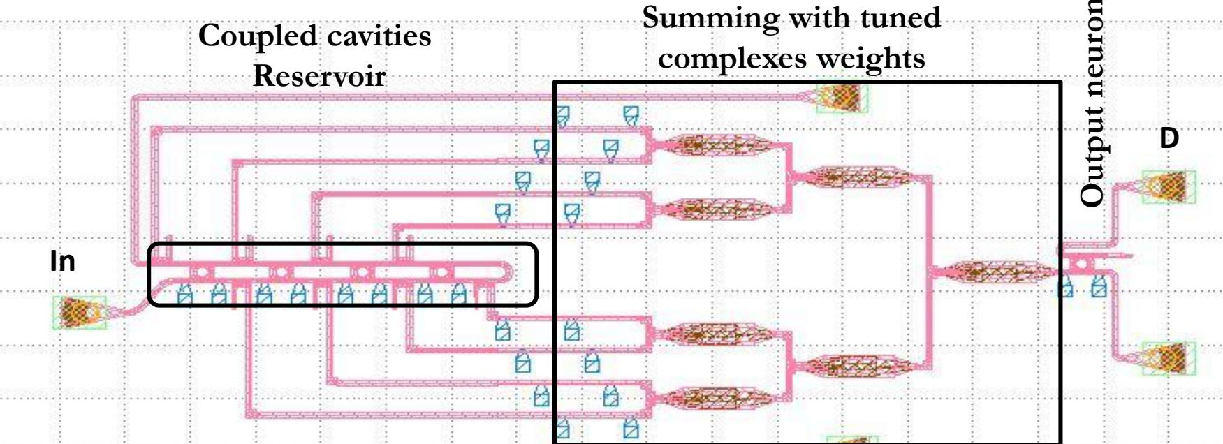
The reservoir is an optical cavity composed by series of coupled ring resonators
